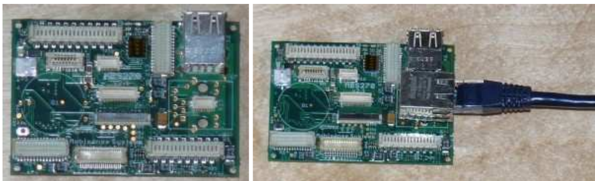
Figure 5: MBS270L without and with RJ45 plug
